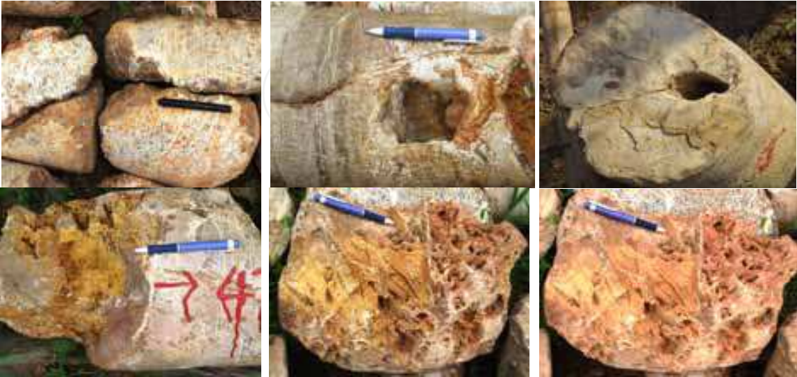
Fig. 5. Corrosion of rock core samples
