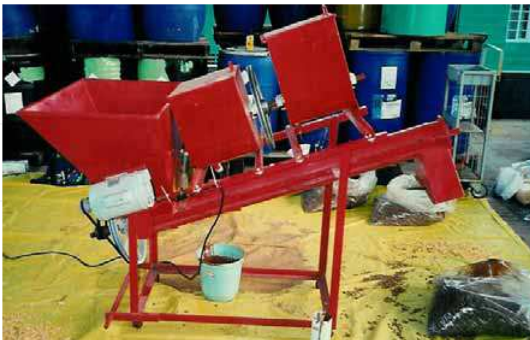
Fig. 18. Seed treatment machine, used to test the application of camouflage in corn seeds. On the floor, in plastic sacks, results of three tests of camouflage by varying the amount of carbofuran syrup, dye powder and water.
