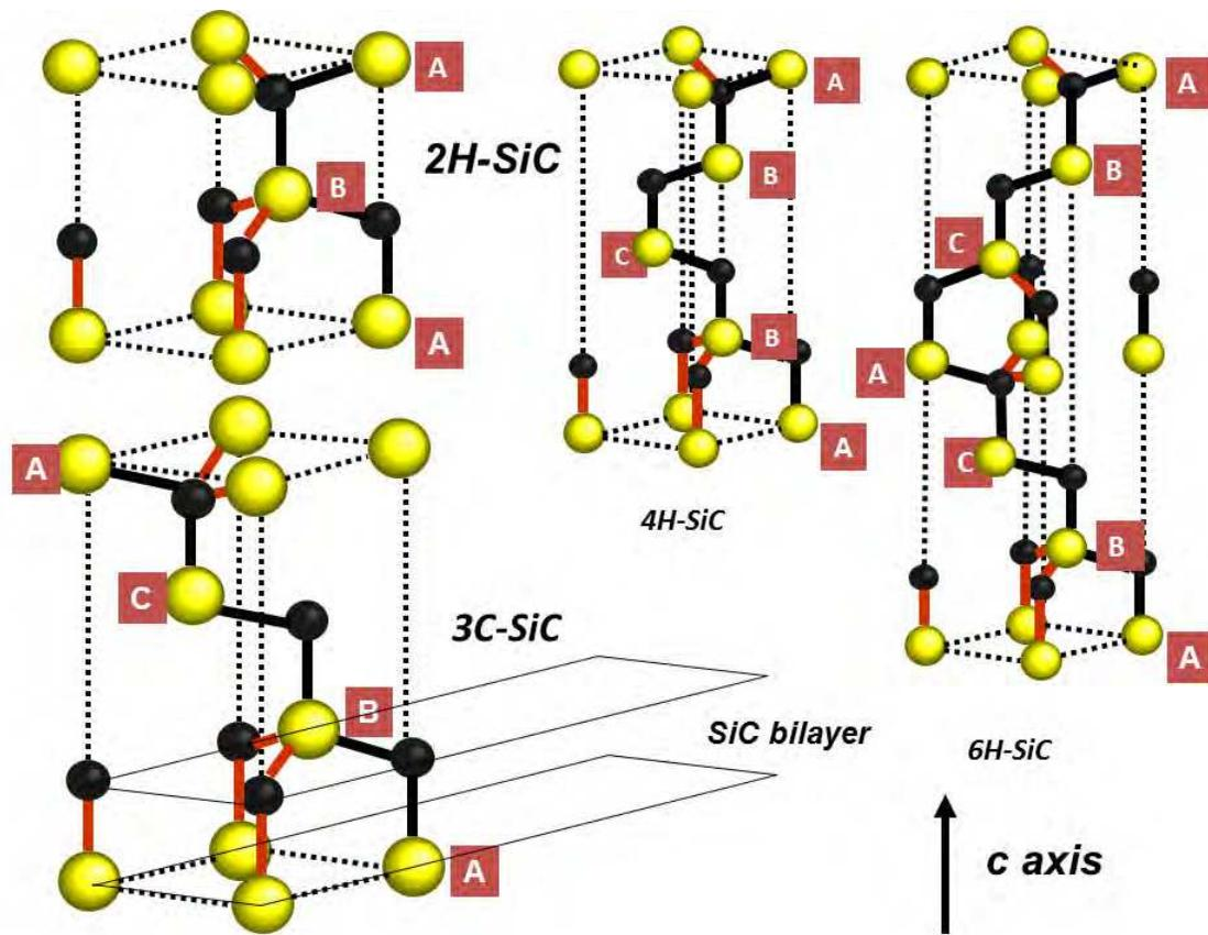
Fig. 5. ball and stick representation in three dimensional perspective of the first polytypes *2H-SiC*, *4H-SiC* and *6H-SiC* compared to *3C-SiC*. The chains structures which defined the stacking sequence are in dark color while selected *Si-C* bonds are in red color. The *SiC* bilayer is also shown. (Kackell, 1994a) after the original figure in reference (Melinon and Masenelli, 2011)
