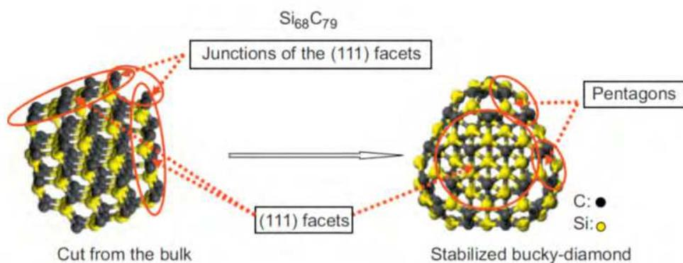
Fig. 8. A piece of  $\beta$  – SiC (truncated octahedron with (111) facets) and the final geometry after relaxation. The more spherical shape indicates a massive reconstruction of the surface. The inner shell remains  $sp^3$  hybridized with a nearly  $T_d$  symmetry while the surface presents a set of pentagons and hexagons which is common in fullerenes. The original figure is in reference (Yu et al., 2009)
