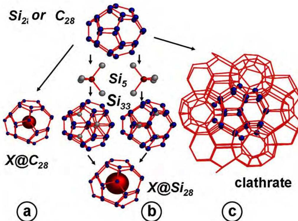
Fig. 7. scenario the an efficient doping in  $C_{28}$  and  $Si_{28}$  cage. Contrary to carbon, silicon needs a giant tetravalent atom. (a) endohedrally doped  $C_{28}$  cage stable for a tetravalent atom (uranium for example). (b) endohedral doping in  $Si_{28}$  cage by incorporation of two  $Si_5$  clusters. The two isomers have roughly the same cohesive energy within DFT-GGA framework. (after the original figure in reference (Melinon and Masenelli, 2009))
