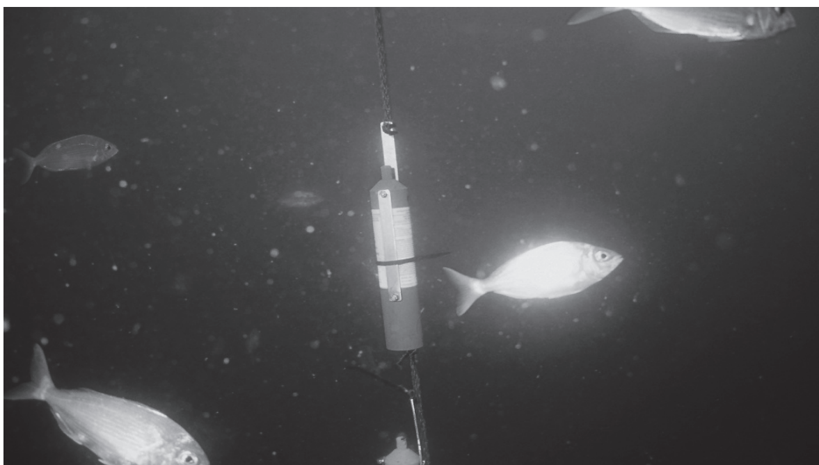
Fig. 2. VR2 receiver deployed in Kromme Bay
