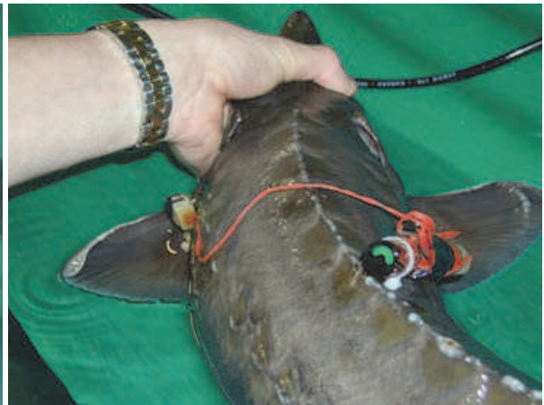
Fig. 48. Tag attached to right pectoral fin and connected to sensor situated on the left pectoral fin.
