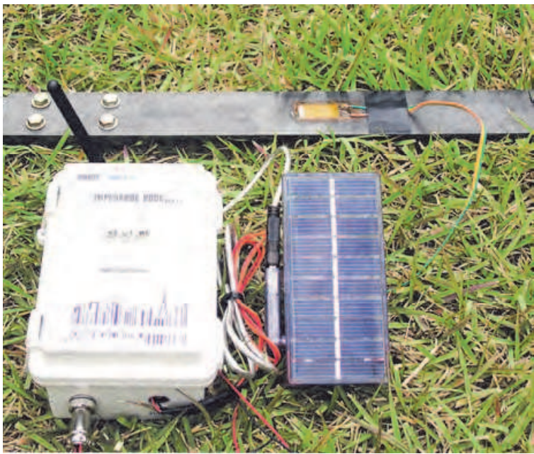
Fig. 6. Sensor node with a solar panel
