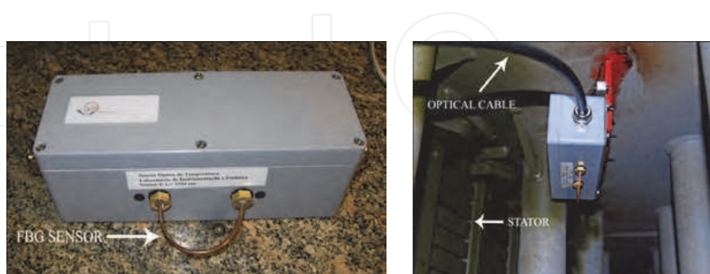
Fig. 3.5.4. Box containing the fiber-optic splices with the FBG inside the U-shape copper tubing (left) and installed inside the generator (right).
