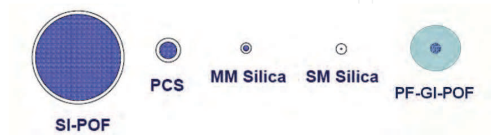
Fig. 2.1. Relative comparison of diameters in different kinds of fibers. SI-POF=step-index polymeric optical fiber; PCS=plastic cladding silica fiber; MM Silica=multimode silica fiber; SM silica=single mode silica fiber; PF-GI-POF=perfluorinated graded-index POF. The light color represents the cladding and dark color the core.
