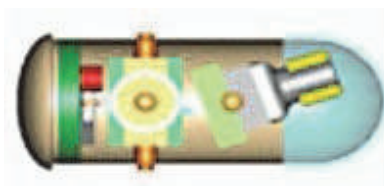
Fig. 12. IVP2 capsule steering system (taken from IVP project website)
