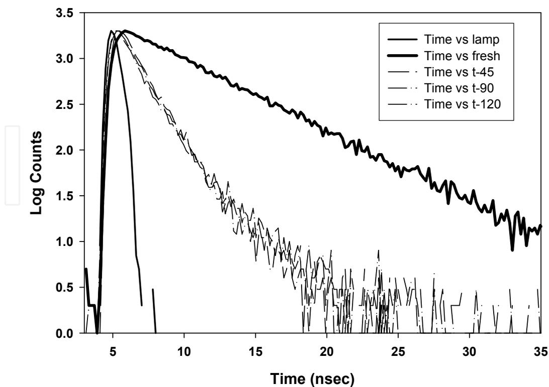
Fig. 7. Fluorescence decay time of fresh and photolyzed samples of  $1 \times 10^{-4} \text{M}$  solutions of benzimidazole in acetonitrile solvent excited at 280 nm.
