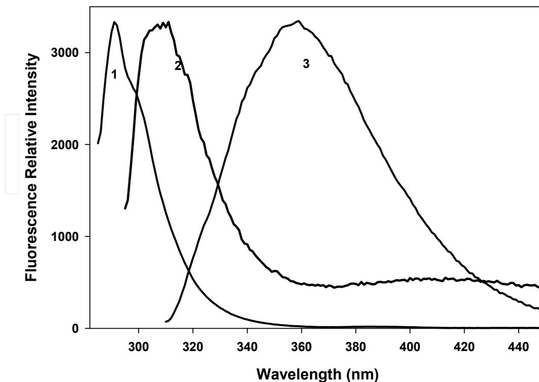
Fig. 3. Fluorescence spectra of fresh samples of  $1 \times 10^{-4}$  M solutions (1) benzimidazole, (2) carbendazim, (3) thiabendazole in acetonitrile solvent. Excitation bands correspond to those obtained from the absorption maxima.
