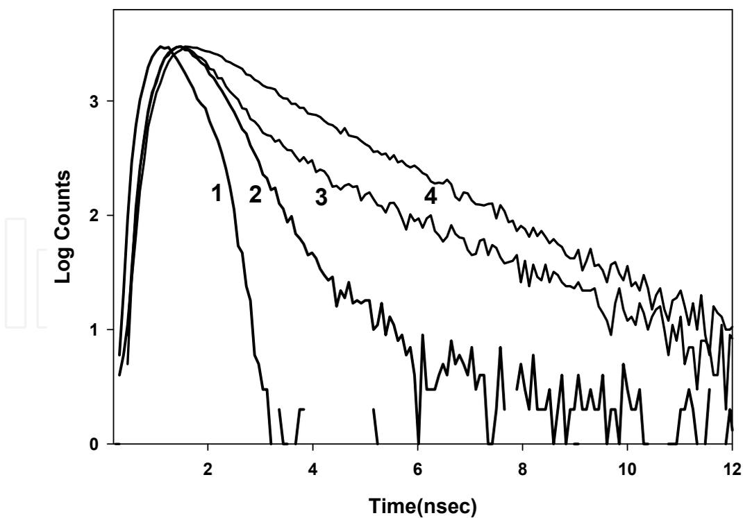
Fig. 10. Fluorescence decay time of fresh and photolyzed samples of  $0.5 \times 10^{-4}$  M solutions of carbendazim in acetonitrile solvent excited at 300 nm. (1) lamp, (2) Fresh, (3) 10 min, (4) 20 min photolysis time.
