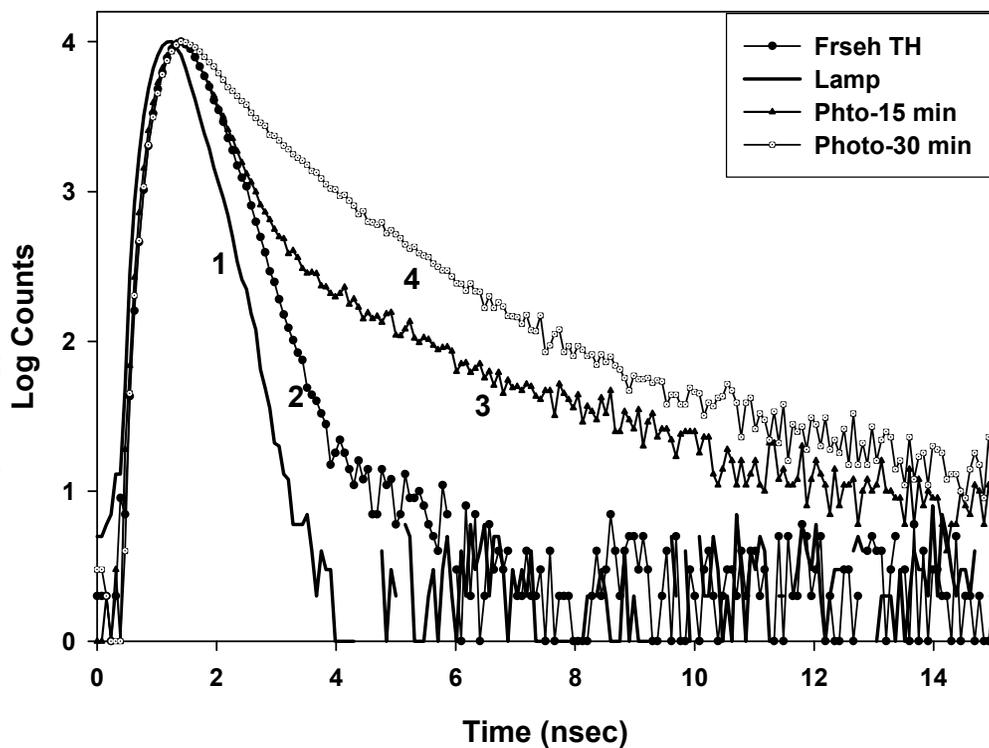
Fig. 13. Fluorescence decay time of fresh and photolyzed samples of  $1.5 \times 10^{-4} \text{M}$  solutions of thiabendazole in acetonitrile solvent excited at 300 nm. (1) lamp, (2) Fresh, (3) 10 min, (4) 20 min photolysis time.
