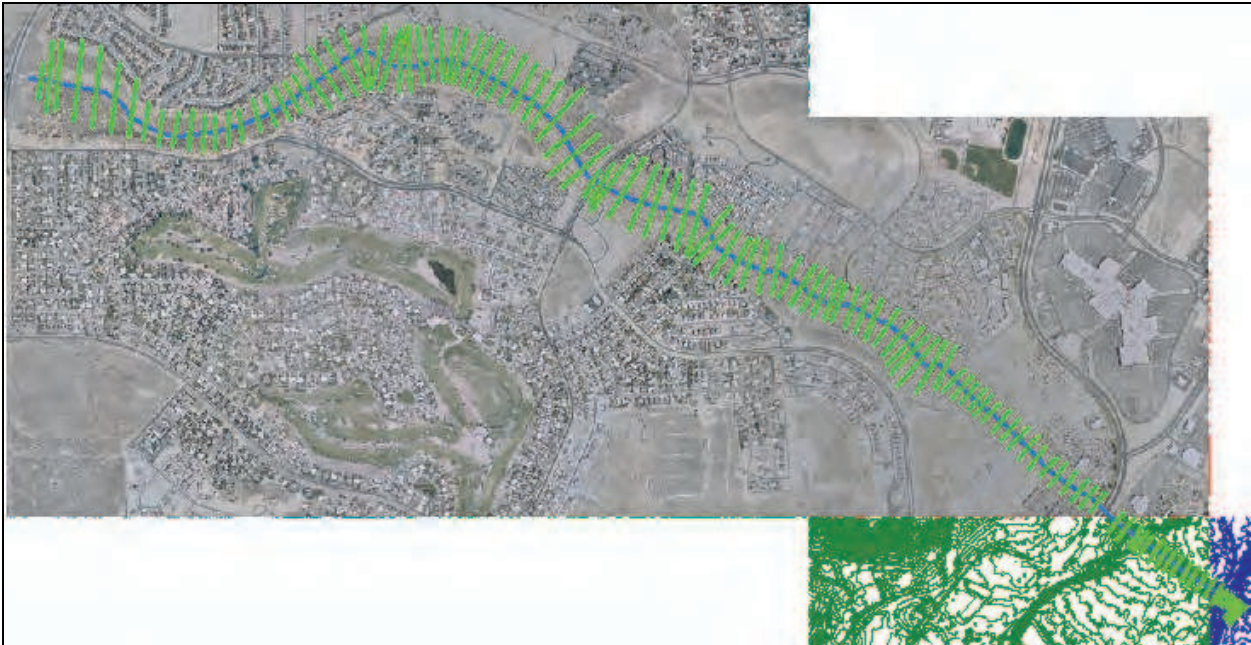
Fig. 4. Image from HEC-GeoRAS showing the cross sections (green lines) and channel centerline (blue line) drawn over the study area. The green and blue contours in the bottom-right show the DTM elevation data processed within ArcGIS.
