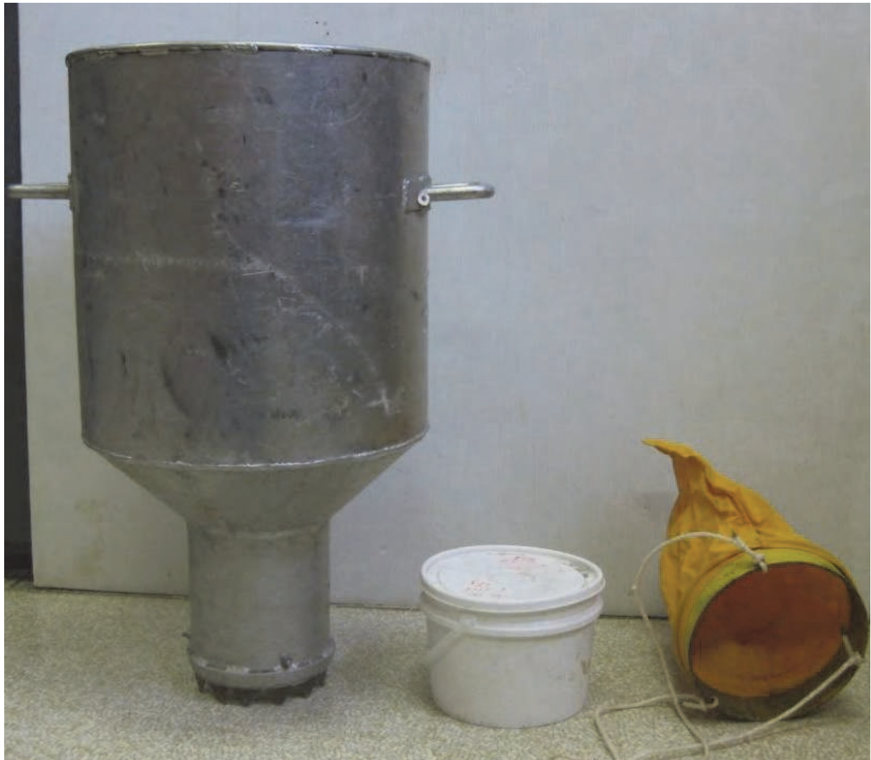
Fig. 1. Laboratory photo of the McNeil corer, gravel bucket, and infiltration bag sampler.
