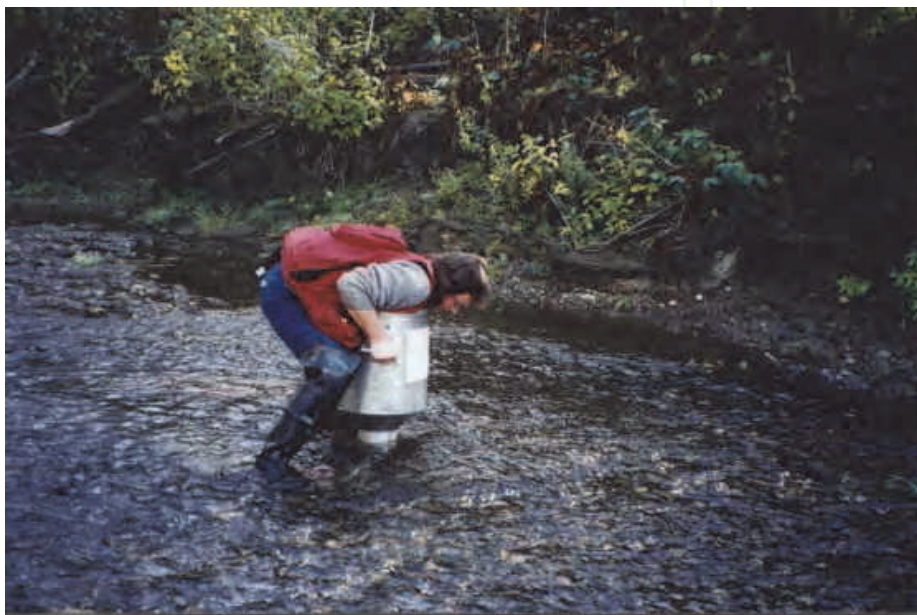
Fig. 4. McNeil core sampling location approached from the downstream direction. The sample is taken by leaning over the core and forcing it into the streambed until it is flush.
