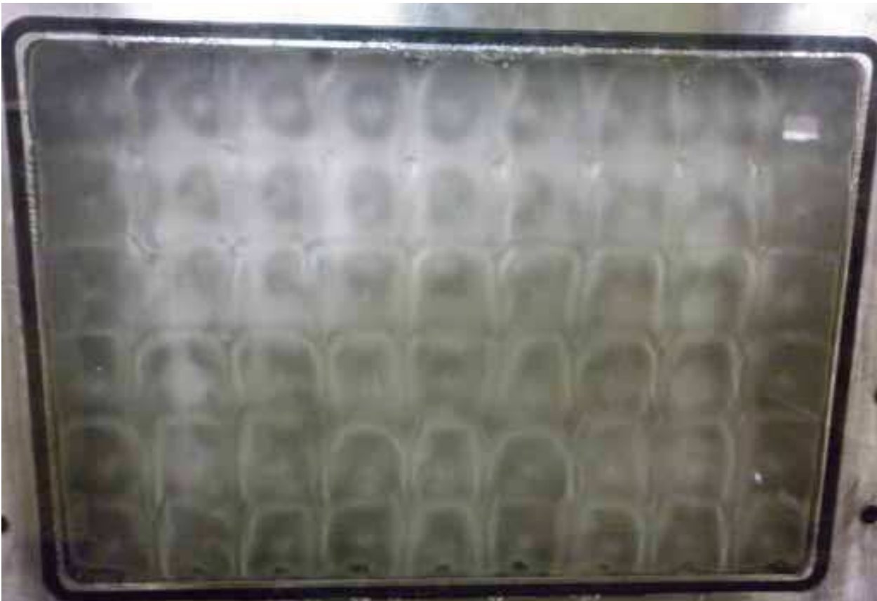
Fig. 20. A transparent surface impinged by a 54-nozzle spray
