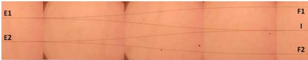
Fig. 37. Coaxial two beam combiner obtained by photographs stitching.
