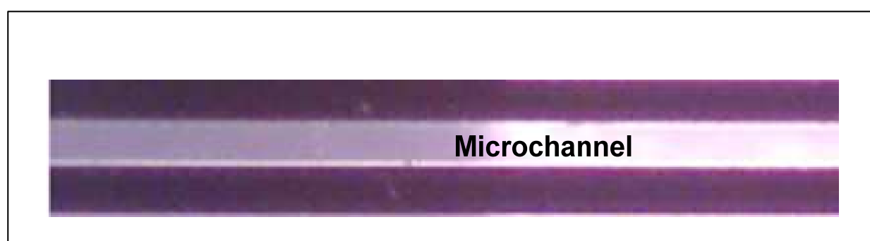
Fig. 1. Color on-line. Photograph (taken under 60 fold magnification) of a wet-etched microfluidic channel on crystalline Si that was used for fabrication of microplasma devices. See text for discussion.
