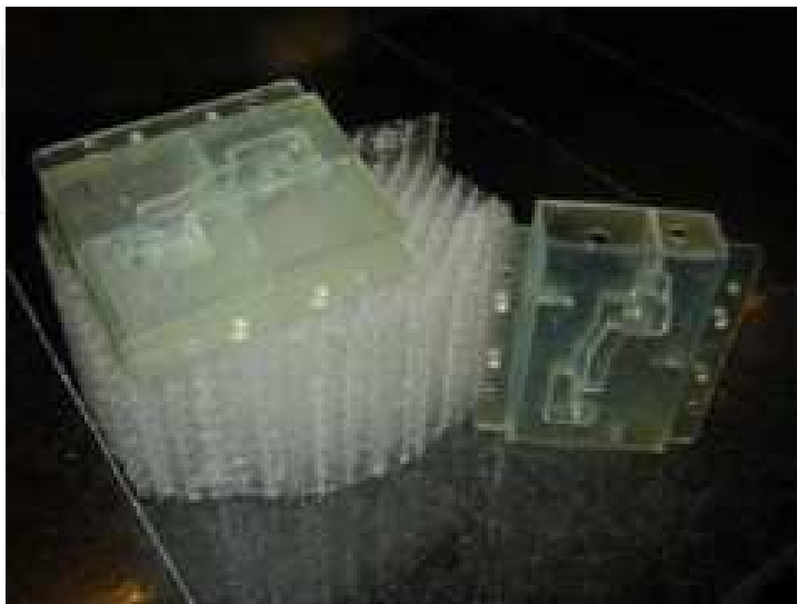
Fig. 21. Fabricated inserts of Peugeot engine gearbox shift fork using stereolithography
