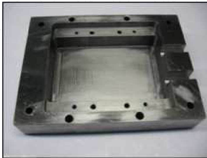
Fig. 22. Base plate machined into a rectangular pocket
