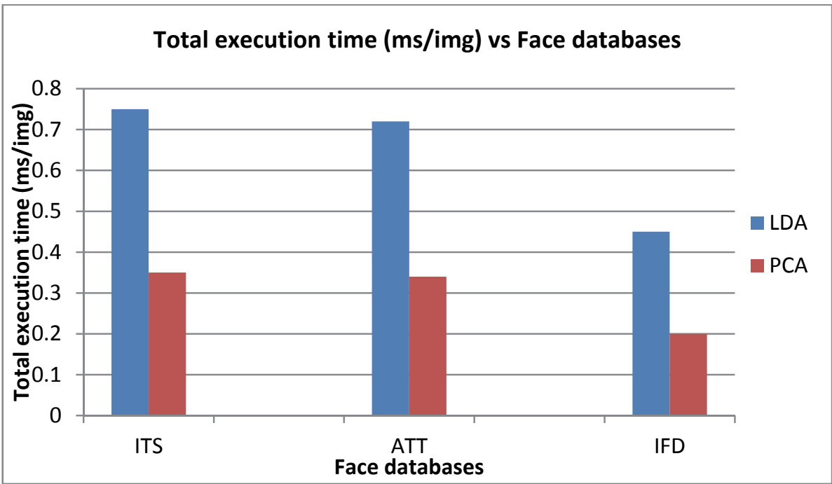
Fig. 5. For total execution time, we can see the Indian face database (IFD) is shortest because the size of each image is lowest then ITS and ATT.
