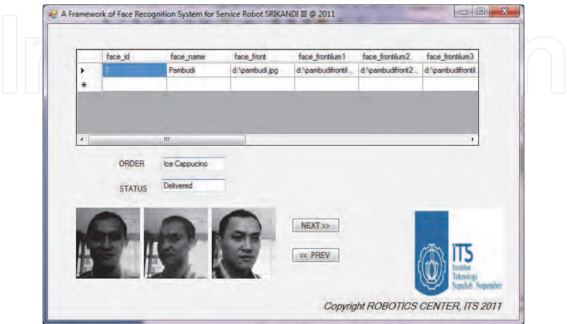
Fig. 3. We have proposed face databases using 1 table, 3 images used for each person (frontal, left and right poses). We have identified the effect varying illumination to the accuracy of recognition for our database called ITS face database as shown in table 1 :
