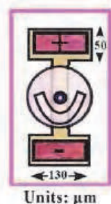
Fig. 15. Bottom-emitting Raycan VCSEL chip
