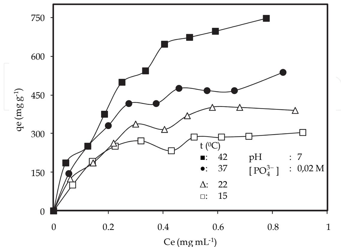
Fig. 8. The effect of temperature on catalase adsorption onto sepiolite
