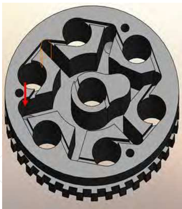
Fig. 14. Plate of oxidizer. Red arrow - inlet of gas.
