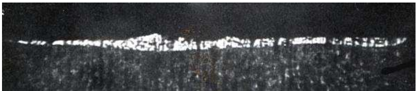
Fig. 8. Metallographic cross-section of laser irradiated steel sample.
