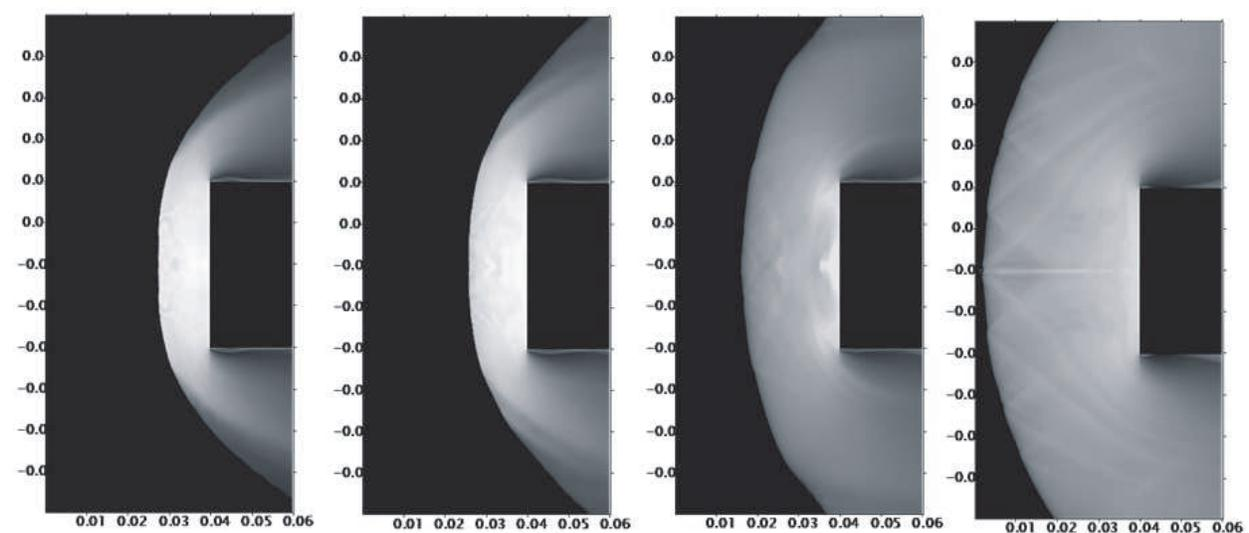
Fig. 9. Flow field calculation for different discharge energy deposition. a) discharge is OFF; b)  $E = 0.044$  eV/mol; c)  $E = 0.049$  eV/mol; d)  $E = 0.054$  eV/mol. Air,  $M = 8.2$ ,  $T_0 = 300$  K,  $P_0 = 35$  Torr,  $T_1 = 21$  K,  $P_1 = 5 \cdot 10^{-3}$  Torr [Khorunzhenko et al, 2003].
