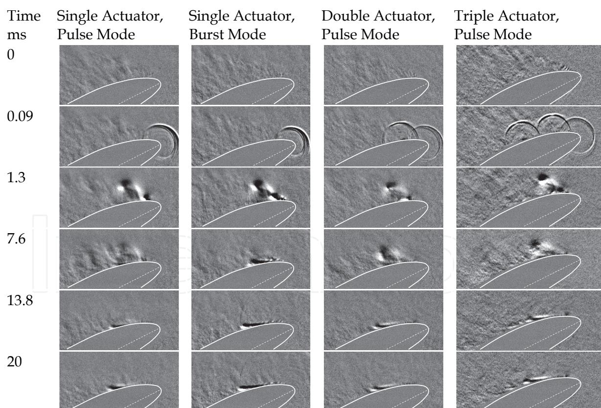
Fig. 39. Dynamics of boundary layer re-attachment.  $V = 30$  m/s,  $\text{AoA} = 26^\circ$ , NACA 63-618 airfoil, chord length was 20 cm wing span was 40 cm. Discharge energy 5 mJ/pulse, discharge frequency 200 Hz in pulse and burst modes; 10 pulses per burst;  $d\tau = 100 \mu\text{s}$  [Correale et al, 2011].
