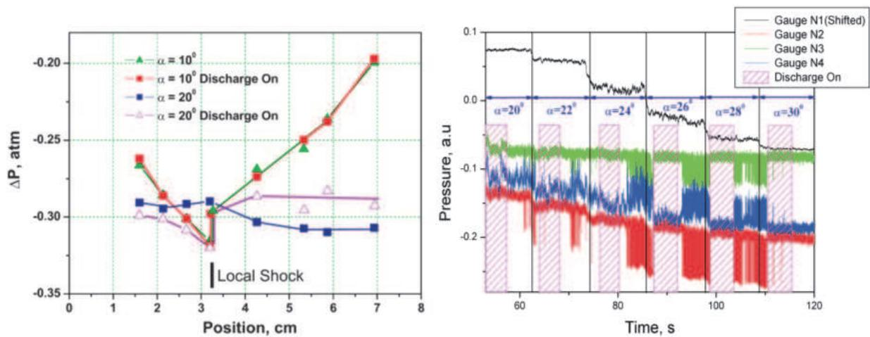
Fig. 38. a) Pressure distribution on model surface with and without discharge. Mach number  $M = 0.74$ . Total pressure  $P = 1$  atm. b) Noise reduction in the wake of the model. Mach number  $M = 0.7$ . Total pressure  $P = 1$  atm [Roupassov et al, 2007].
