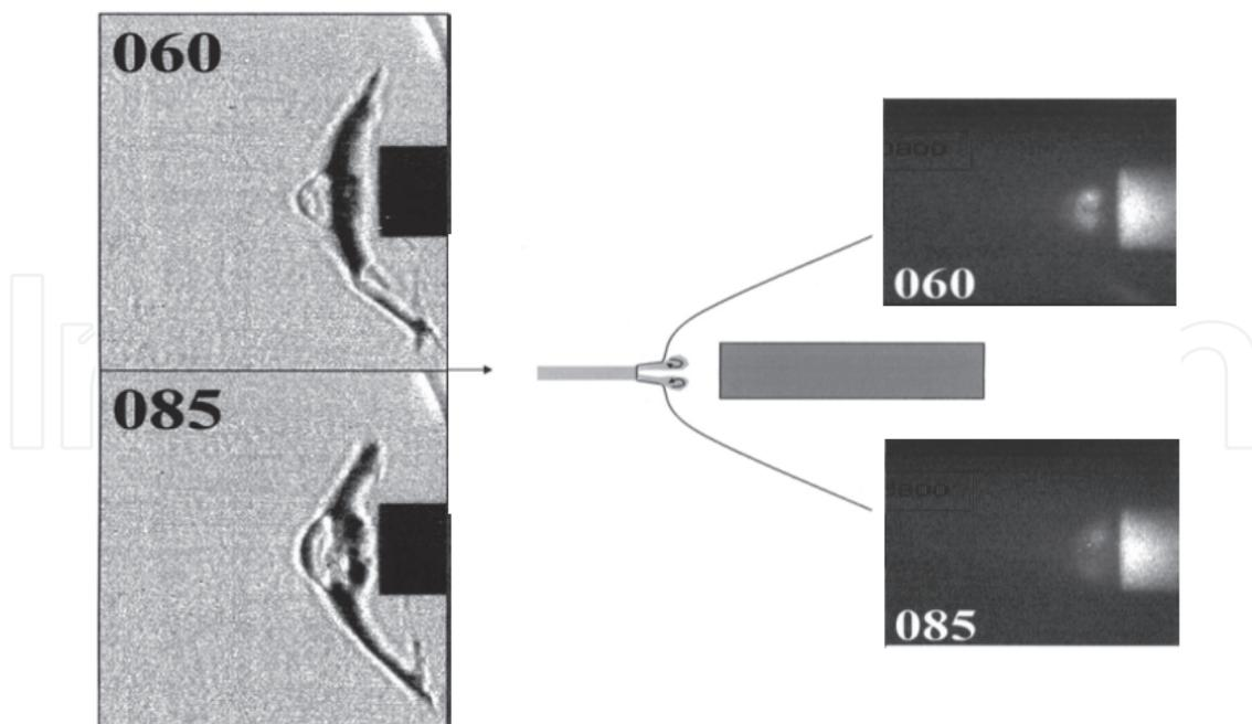
Fig. 15. Interaction of microwave filament with blunt body flow. Left - Schlieren images; right - luminosity distribution fields. 60 and 85  $\mu$ s after the MW discharge [Kolesnichenko et al, 2004].
