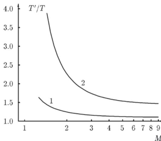
Fig. 11. Dependence of the critical layer overheating  $(T/T')_{crit}$  on the shock wave Mach number.  $\gamma = 1.4$ . 1) - Mark-Griffiths criterion, 2) - modified criterion [Lashin&Starikovskii, 1995].
