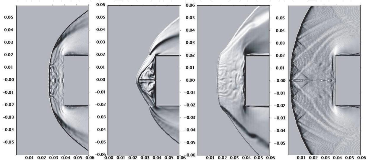
Fig. 12. Numerical model of hot layer – shock wave interaction. The influence of layer thickness. Air,  $M = 8.2$ ,  $T_0 = 300$  K,  $P_0 = 35$  Torr. Excitation energy is  $E = 0.054$  eV/mol, layer thickness is a) 0%; b) 10%; c) 100% and d) entire flow [Opaits et al, 2004].
