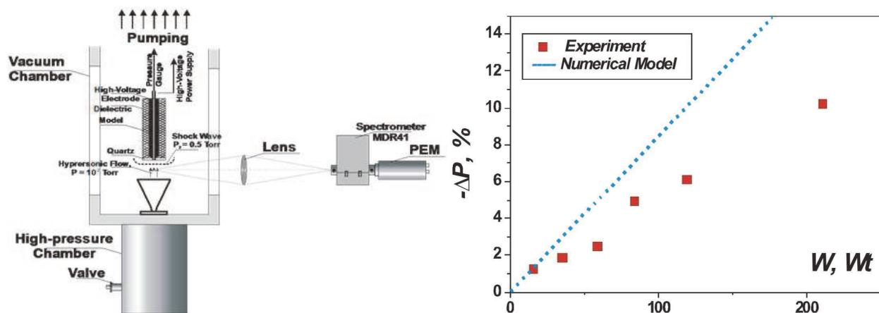
Fig. 8. a) Organization of hypersonic plasma flow. b) Comparison of the experimental results and numerical modeling of stagnation pressure variation vs discharge power in  $M = 8.2$  air flow [Khorunzhenko et al, 2003].
