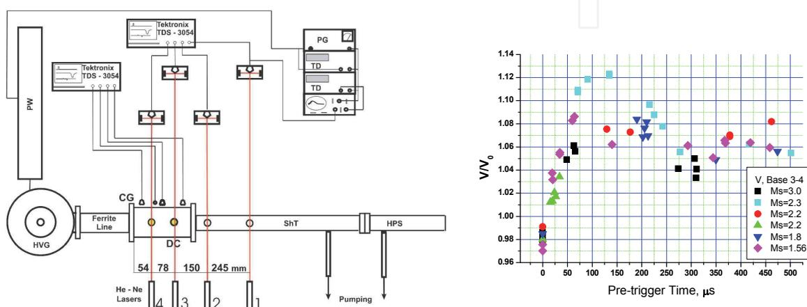
Fig. 10. Plasma shock tube schematics a) and shock wave acceleration in the plasma region in dependence on the plasma relaxation time [Anokhin et al, 2004].
