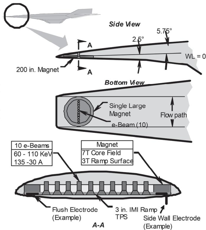
Fig. 23. MHD inlet control system [Van Wie, 2004].
