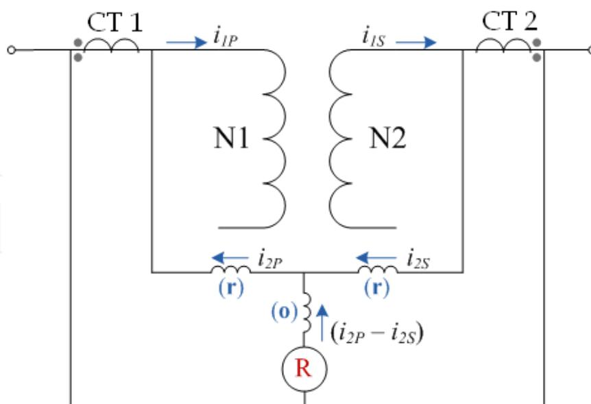
Fig. 3. Differential relay connections.
