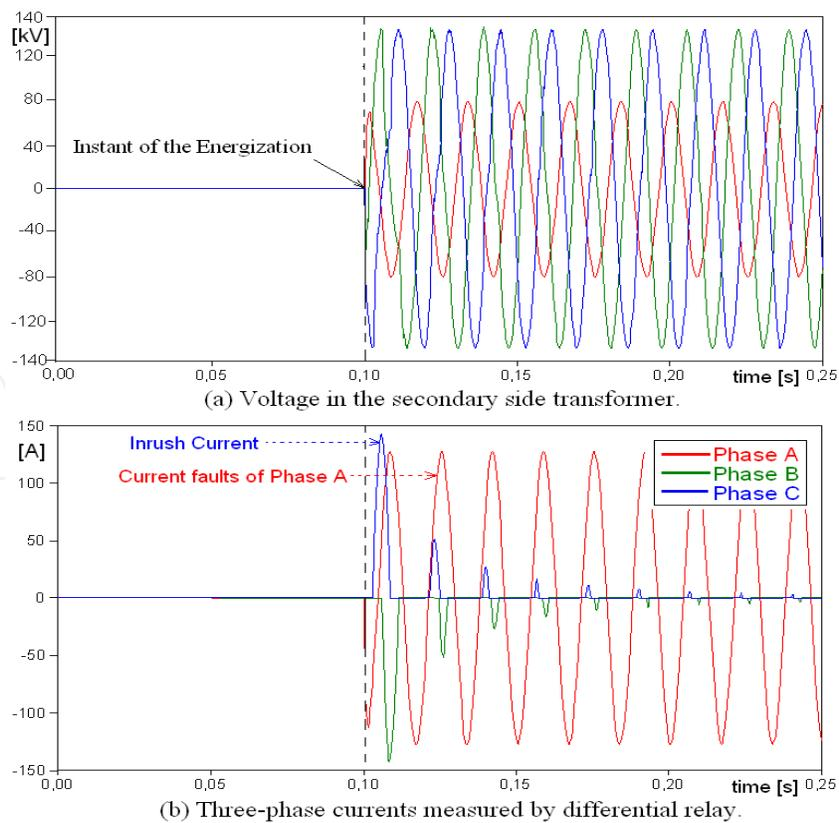
Fig. 8. Energization and internal faults simulation on PT.
