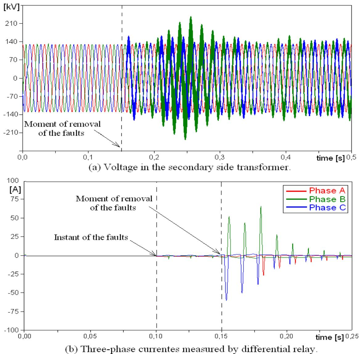
Fig. 9. External faults removal simulation.
