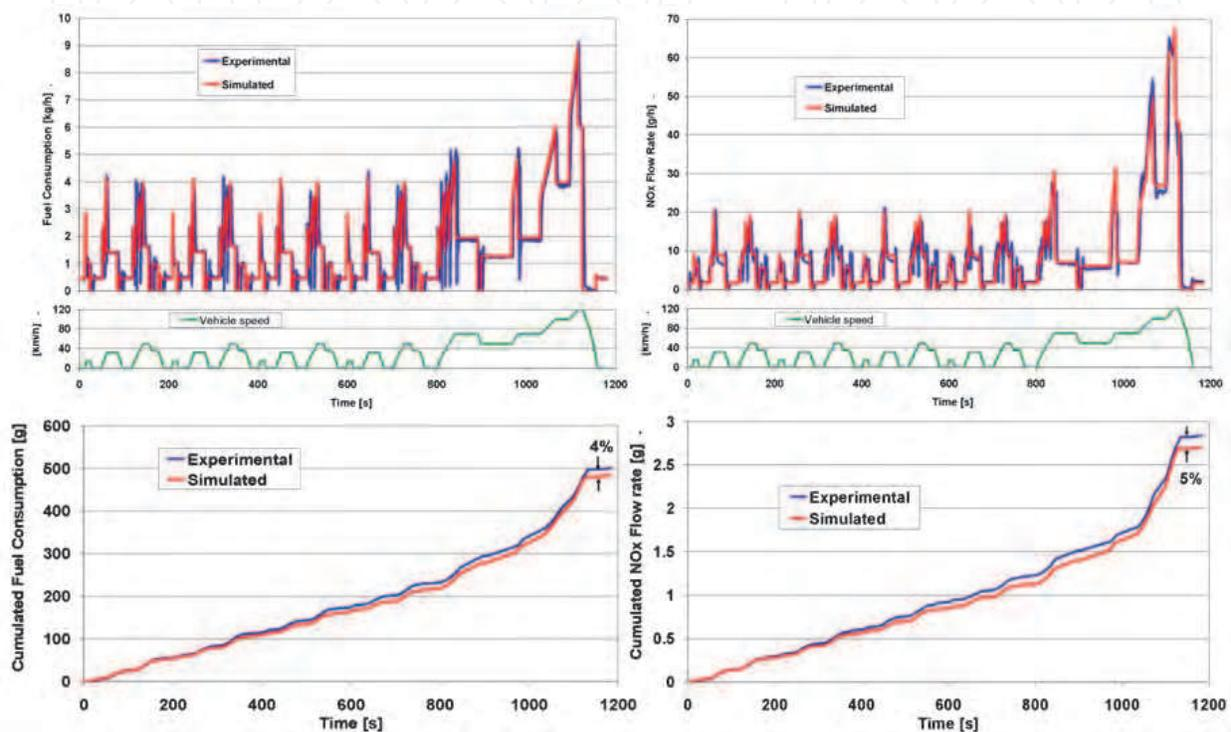
Fig. 4. Top: fuel consumption and NO<sub>x</sub> emission rate over warm NEDC cycle for a conventional powertrain. Bottom: cumulated fuel consumption and NO<sub>x</sub> emissions on the same driving cycle (from Vassallo et. al., 2007).
