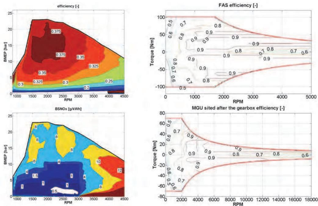
Fig. 15. Performance Maps – Left: Engine Efficiency and BSNOx maps. Right: MGUs efficiency maps.
