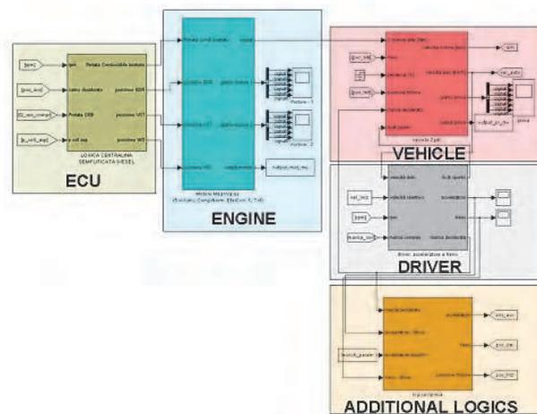
Fig. 10. Simulink vehicle mean value model: global layout
