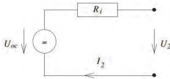
Fig. 9. Battery static model
