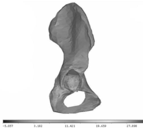
Fig. 12. 1<sup>st</sup> principal stress for extension
