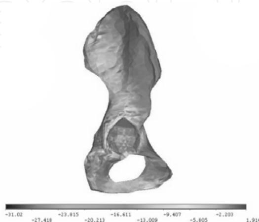
Fig. 13. 3<sup>rd</sup> principal stress for extension
