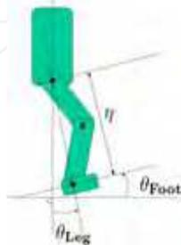
Figure 6. Kinematic interface to a leg
