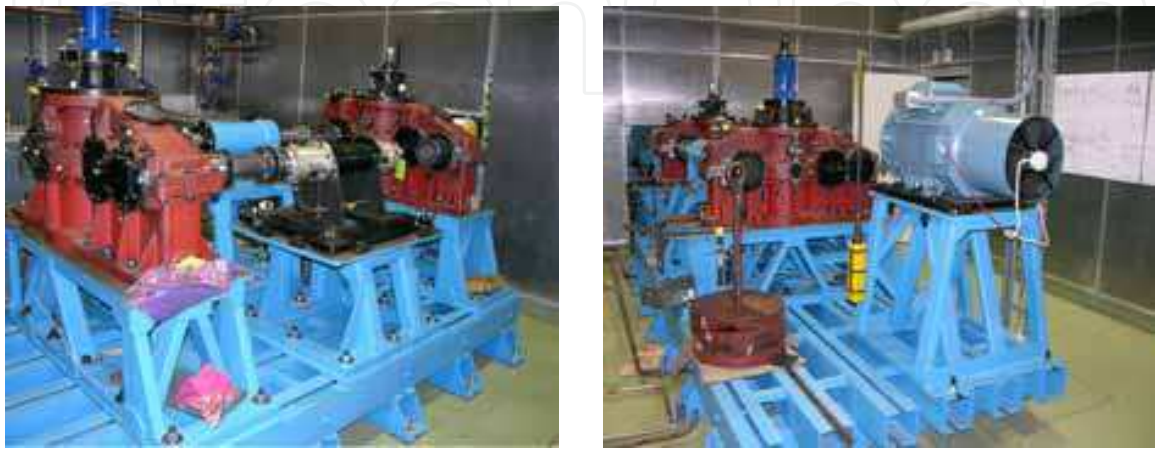
Fig. 3. Gear fatigue test rig overall view
