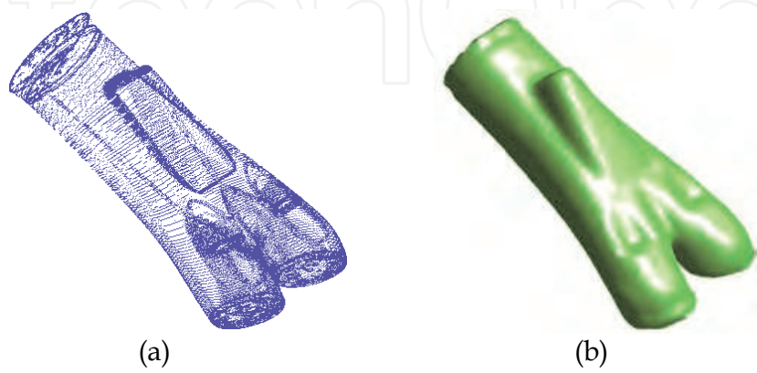
Fig. 15. Reconstruction of engine outtake ports. (a) Point clouds and details. (b) Final resulting surface and details.
