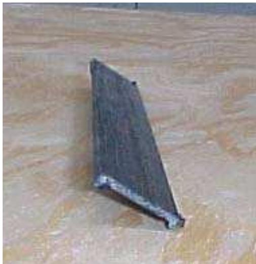
Fig. 19. U-Shape GF/PP pultruded profile made from towpregs
