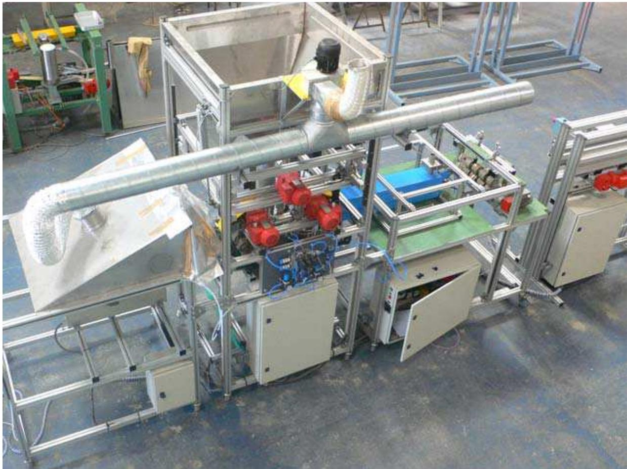
Fig. 2. Powder coating equipment
