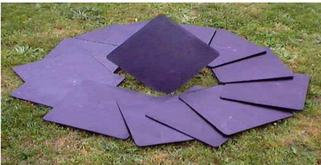
Fig. 20. GF/PP LFT plates made from towpregs
