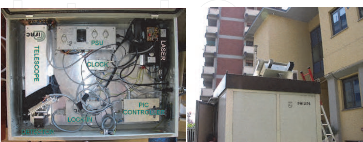
Fig. 12. The instrument opened (left) and installed on the roof of the ARPAT, PM-monitoring station in Florence (I) (right)
