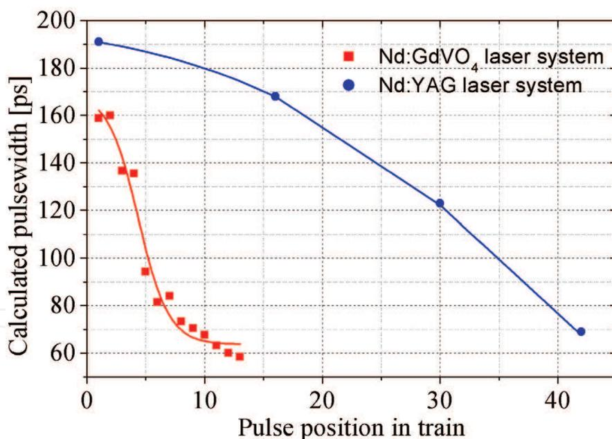
Fig. 7. Calculated pulse duration evolution along the trains generated by the Nd:GdVO<sub>4</sub> and Nd:YAG laser systems.
