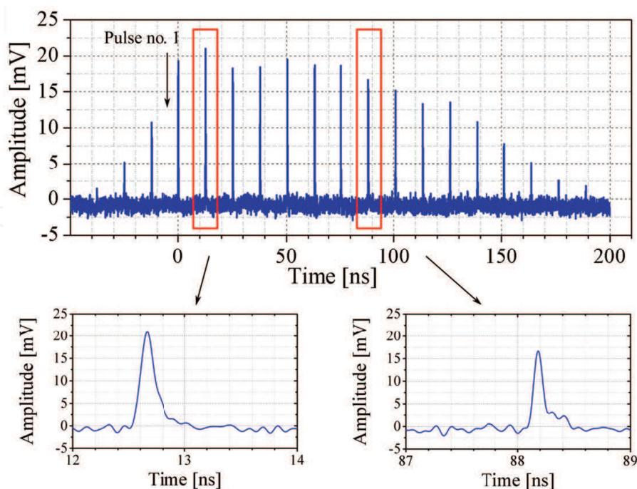
Fig. 6. Nd:GdVO<sub>4</sub> laser system output pulse train oscillogram (upper trace) and zoomed pulses no. 3 and 9 (lower traces).
