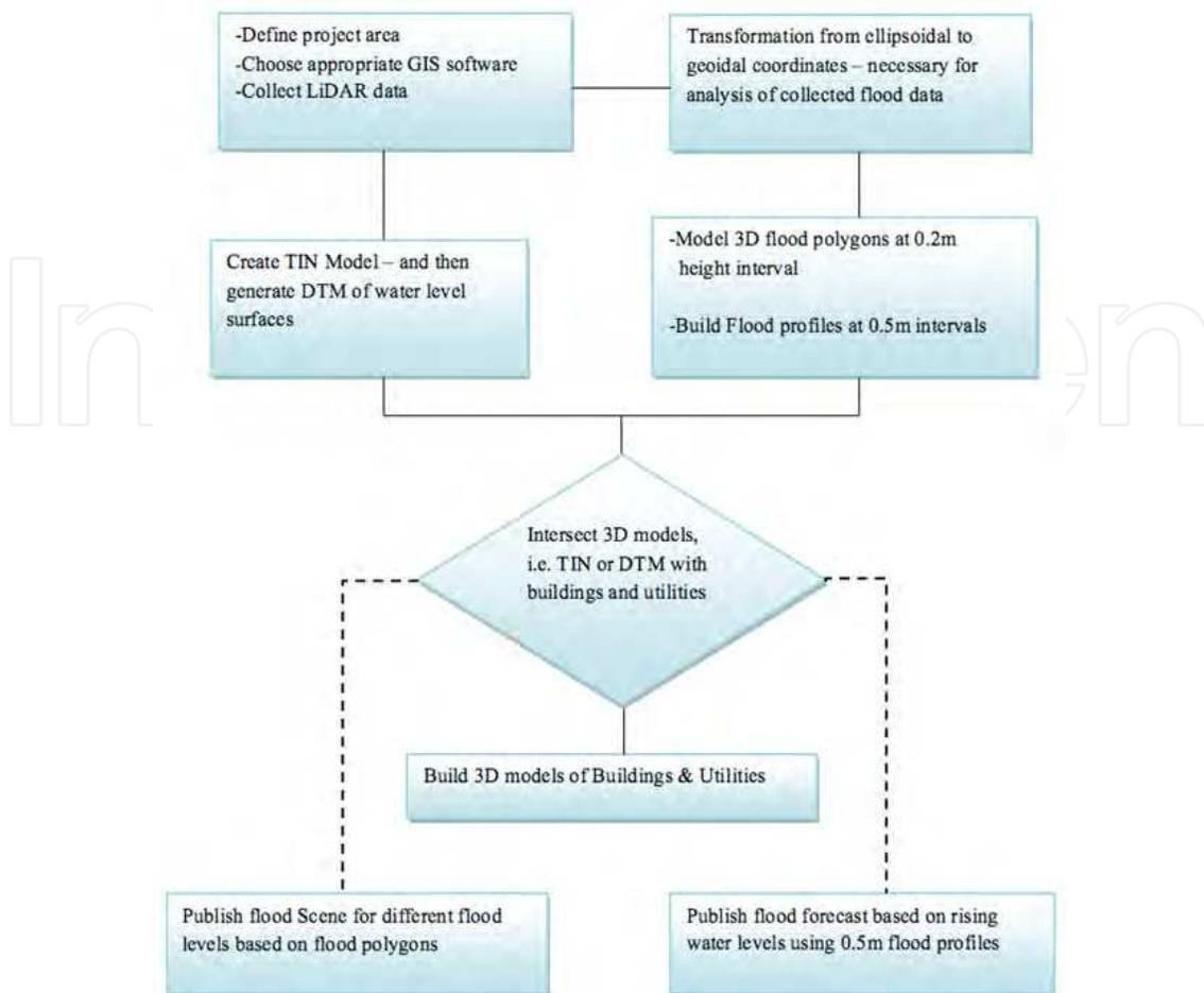
Fig. 11. The workflow of detailed methods and techniques applied for modelling of flooded buildings and infrastructure.
