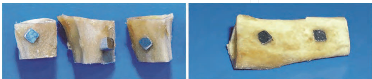
Fig. 5. The biological materials aspect after sampling: left-Ti 99,99% at 2, 4 and 6 months after implantation; right Ti6Al4V and 316L respectively, two months after implantation.
