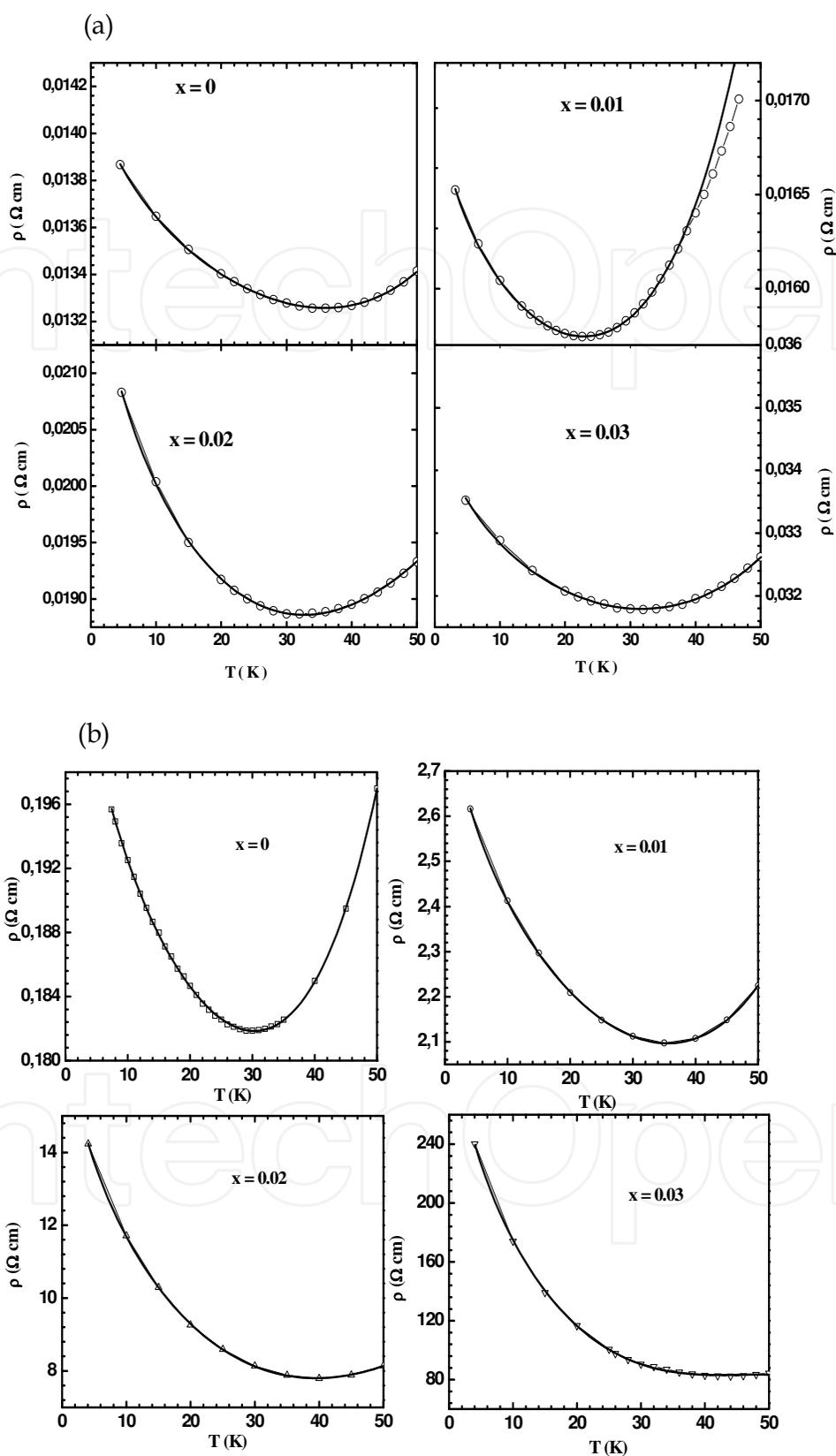
Fig. 7. Electrical resistivity variation with temperature below 50K (a)  $La_{2/3}Ba_{1/3}(Mn_{1-x}Sb_x)O_3$  and, (b)  $Pr_{2/3}Ba_{1/3}(Mn_{1-x}Sb_x)O_3$  ( $0 \leq x \leq 0.03$ ). Solid line shows the fitting with the Eq. (3).
