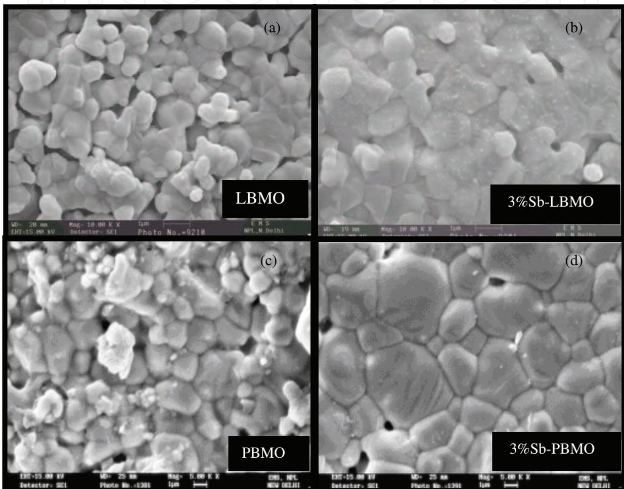
Fig. 5. SEM micrographs of (a)  $\text{La}_{2/3}\text{Ba}_{1/3}\text{MnO}_3$ , (b)  $\text{La}_{2/3}\text{Ba}_{1/3}\text{Mn}_{0.97}\text{Sb}_{0.03}\text{O}_3$  (3Sb-LBMO), (c)  $\text{Pr}_{2/3}\text{Ba}_{1/3}\text{MnO}_3$ , (d)  $\text{Pr}_{2/3}\text{Ba}_{1/3}\text{Mn}_{0.97}\text{Sb}_{0.03}\text{O}_3$  (3Sb-PBMO).
