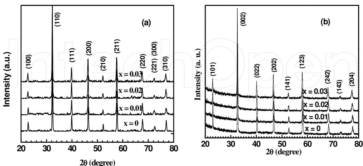
Fig. 4. X-ray diffraction patterns of (a)  $\text{La}_{2/3}\text{Ba}_{1/3}(\text{Mn}_{1-x}\text{Sb}_x)\text{O}_3$  and (b)  $\text{Pr}_{2/3}\text{Ba}_{1/3}(\text{Mn}_{1-x}\text{Sb}_x)\text{O}_3$  ( $0 \leq x \leq 0.03$ ) samples.
