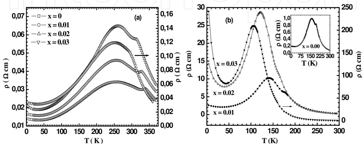
Fig. 6. Electrical resistivity variation with temperature of (a)  $\text{La}_{2/3}\text{Ba}_{1/3}(\text{Mn}_{1-x}\text{Sb}_x)\text{O}_3$  and (b)  $\text{Pr}_{2/3}\text{Ba}_{1/3}(\text{Mn}_{1-x}\text{Sb}_x)\text{O}_3$  ( $0 \leq x \leq 0.03$ ).
