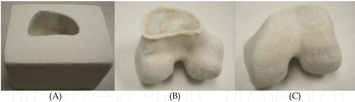
Fig. 27. A: 3-D printed plaster femur head mold; B&C: Front and bottom view of Injected PCL femur head.
