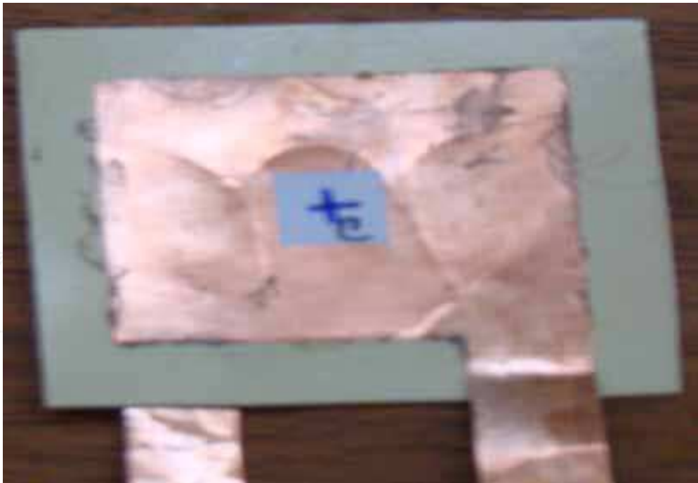
Fig. 12. Composite sample 50 vol% (grey) with cooper foil for electric contact.
