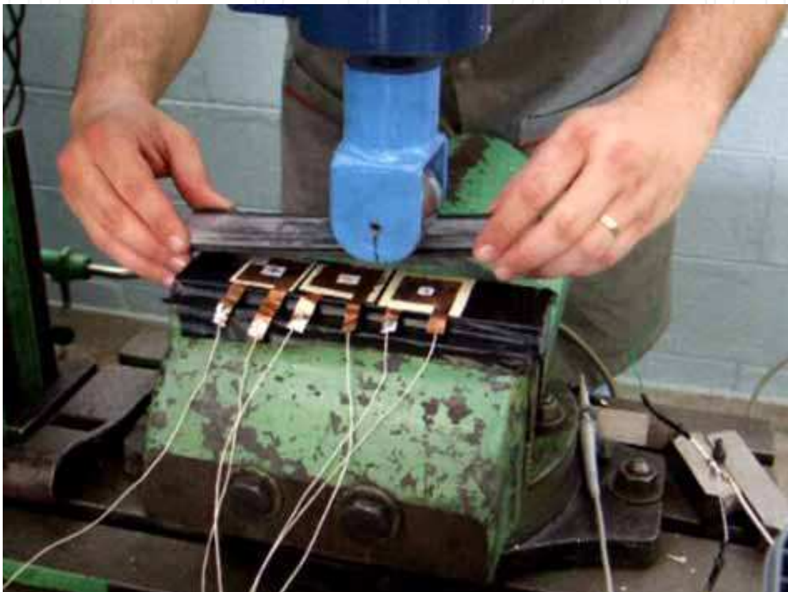
Fig. 13. System used to simulate the vehicle traffic or people walking.
