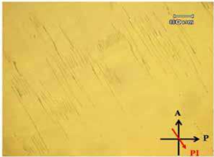
Fig. 4. The SSFLC texture of the FLC+1wt% BaTiO 3 at 30°C, under 200 times POM magnification. (The red arrow indicates the PI alignment rubbing direction)
