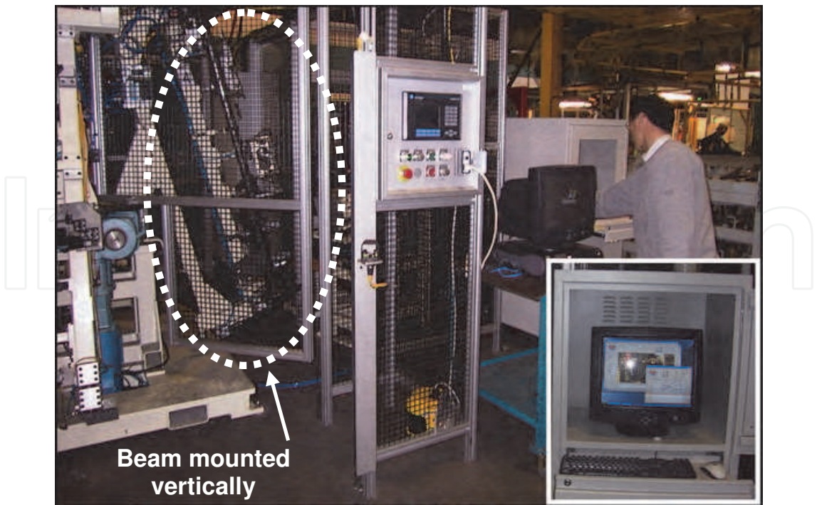
Fig. 3. PLC controlled manufacturing cell with PC controlled vision system.
