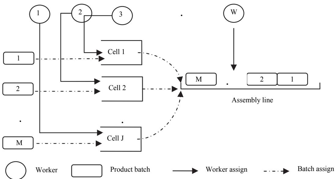
Fig. 1. A hybrid assembly system
