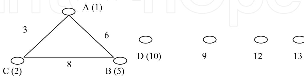
Also three specific 2-factors interactions are investigated through the experiment. Above graph shows the factors (A, B, C and D) and their specific 2-factors (A×B, A×C and B × C) interactions and which column they will be in Appendix 3.
