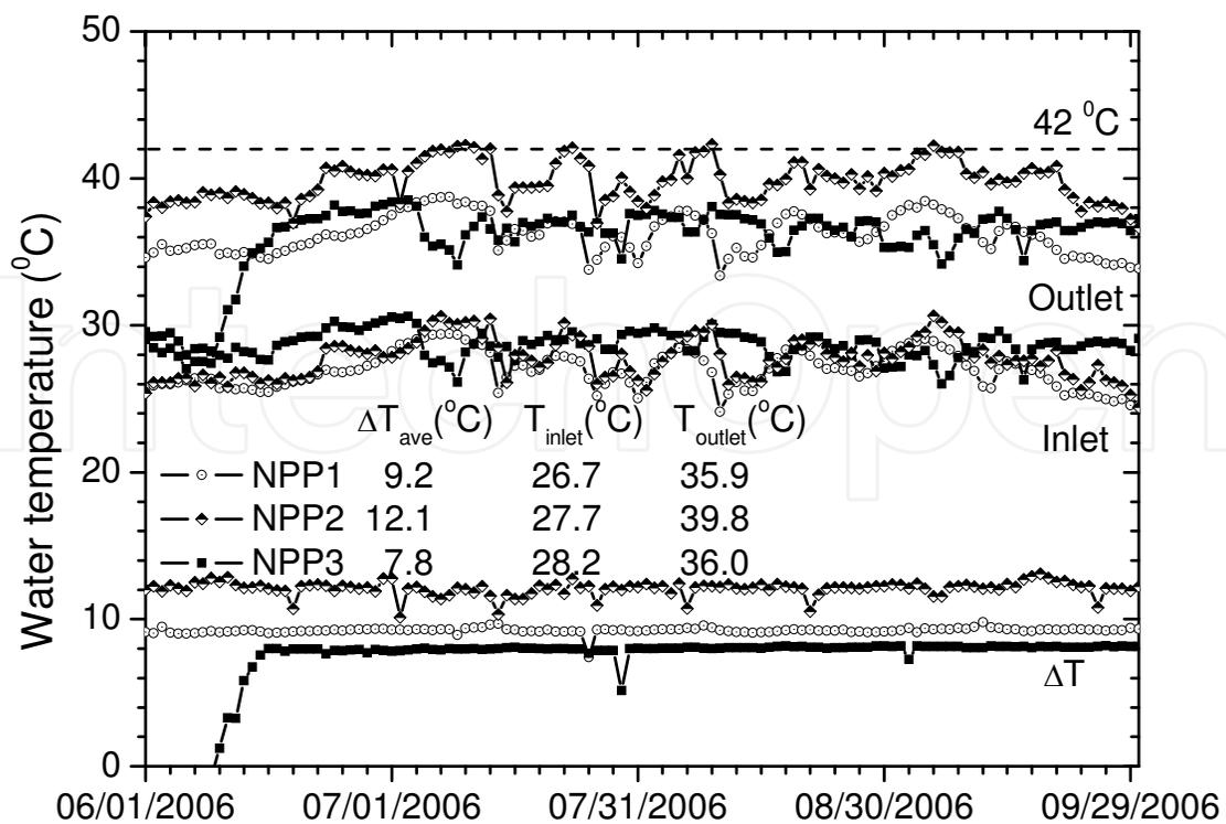
Fig. 4. The average temperature of NPP1, NPP2, and NPP3 at the condenser inlet and outlet from June to September in 2006.  $\Delta T$  is the elevated temperature of cooling water between the condenser inlet and outlet. NPP3 was not operated in full power before June 15
