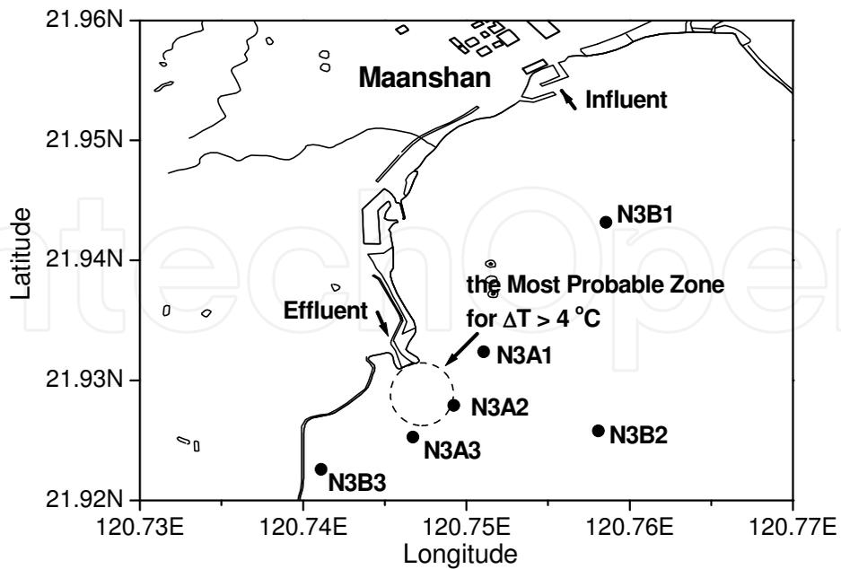
Fig. 9. The locations of water temperature monitors group A, N3A1, N3A2, and N3A3 and corresponding group B, N3B1, N3B2, and N3B3 at NPP3. Group A is 500 m away from the effluent discharge point. Group B is set as the background temperature of marine water
