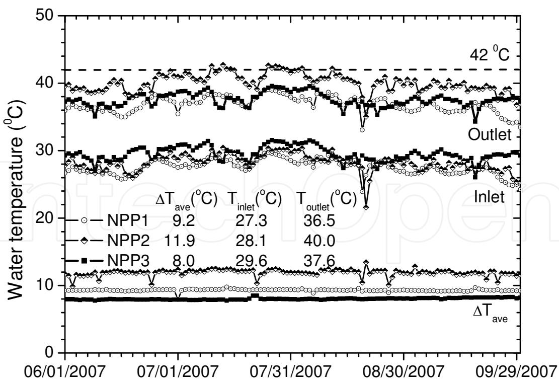
Fig. 5. The average temperature of NPP1, NPP2, and NPP3 at the condenser inlet and outlet from June to September in 2007.  $\Delta T$  is the elevated temperature of cooling water between the condenser inlet and outlet
