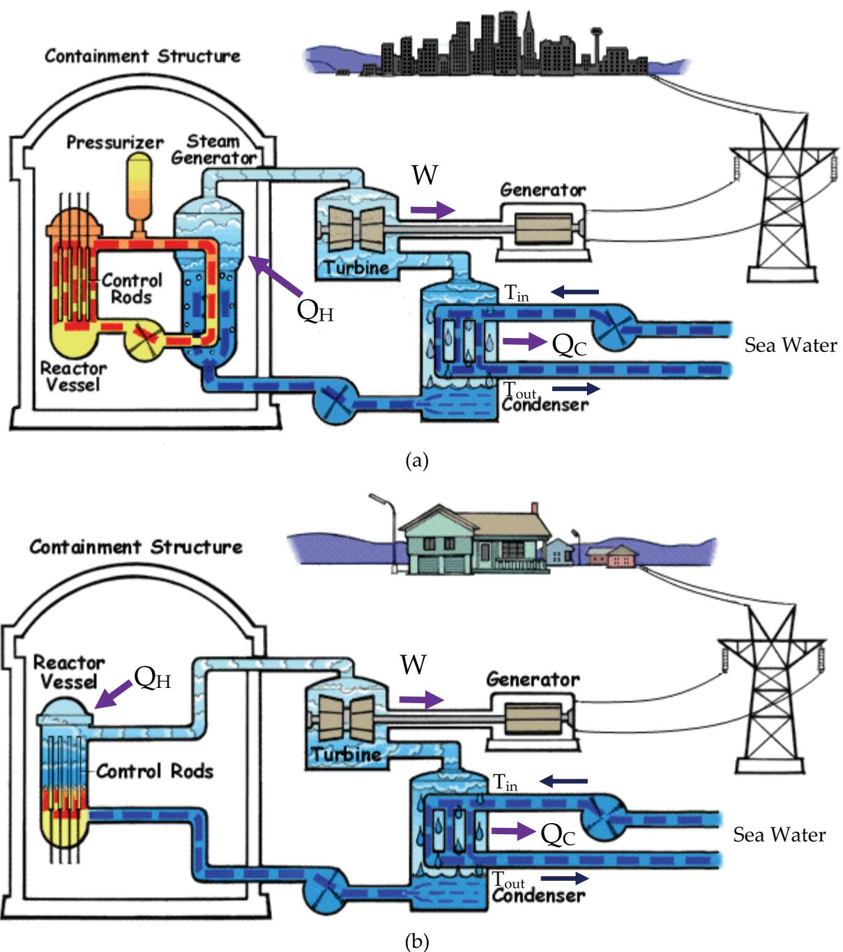
Fig. 3. The schematic diagram of (a) a PWR; (b) a BWR. The heat transfer routes are also depicted, respectively. (background images are taken from USNRC, 2011 b)
