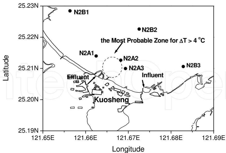
Fig. 8. The locations of water temperature monitors group A, N2A1, N2A2, and N2A3 and corresponding group B, N2B1, N2B2, and N2B3 at NPP2. Group A is 500 m away from the effluent discharge point. Group B is set as the background temperature of marine water
