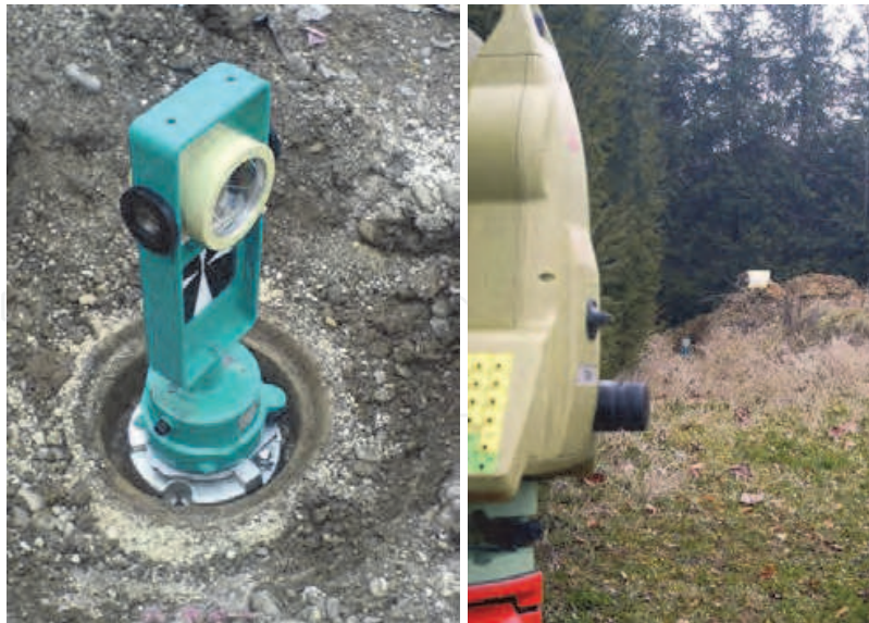
Fig. 3. Signalisation of the centre and the ex-central stand
