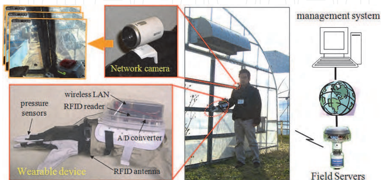
Fig. 3. Overview of the prototype system and the wearable device.
