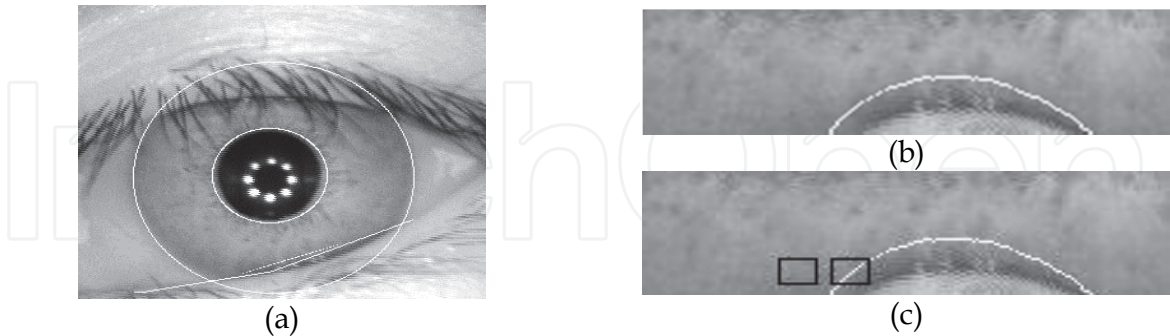
Fig. 8. Illustration of eyelids boundary evaluation (a) segmented iris image (b) segmented RI in polar coordinates (c) selection of two neighbours blocks near and on the detected boundary
