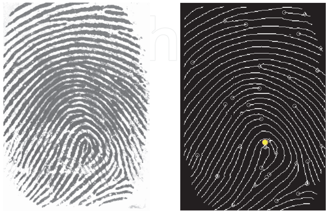
Fig. 7. Fingerprint 101_1 and its enhanced thinned version.
