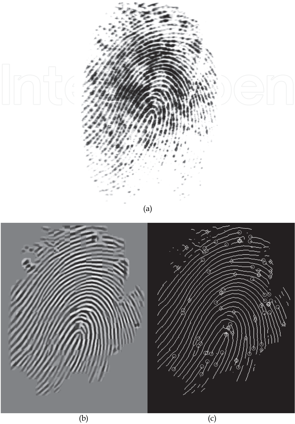
Fig. 6. a) Fingerprint image 108_7 from DB1_B in FVC2000, b) Enhanced version of fingerprint image 108_7, c) core point (asterisk), terminations (circles) and bifurcations (diamonds).
