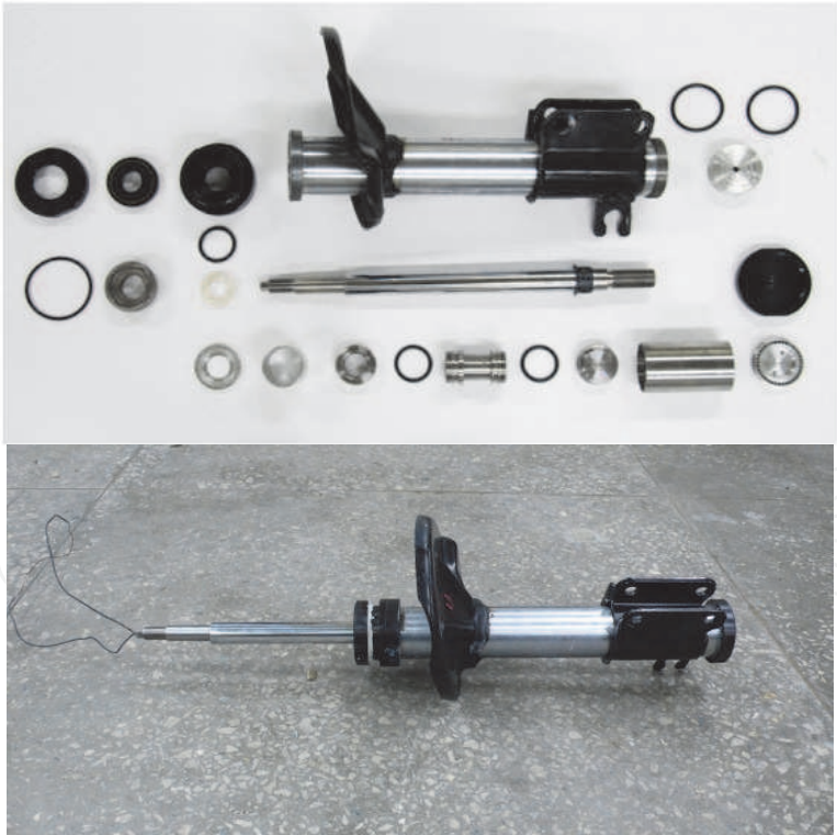
Fig. 3. Photograph of the manufactured MR damper
