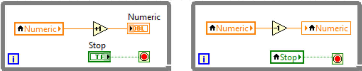
Fig. 3. A simple example of race condition using local variables that are changed in two independently running loops
