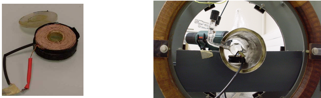
Fig. 5. The transmit-receive coil (left figure). On the right figure, the coil could be seen inside the Helmholtz coils and the shield. The coil is loaded by a sample consisting of Pyrex (a type of glass) cylinder filled with pure water.
