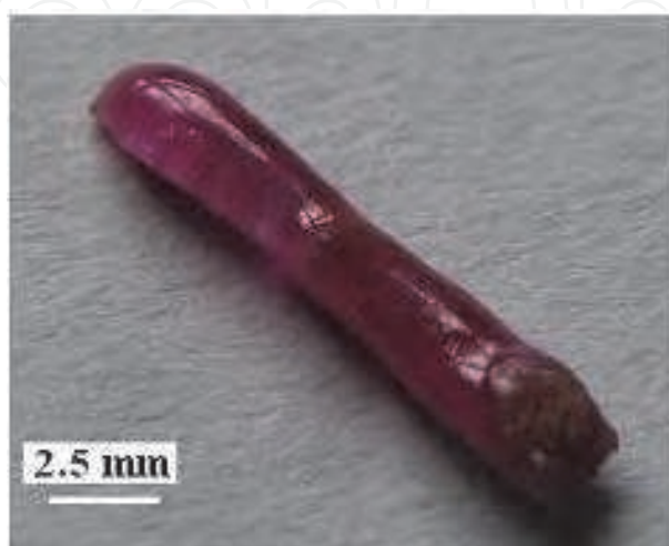
Fig. 13. View of a specimen after laser irradiation at P = 70 W and v = 0.0094 mm/s.
