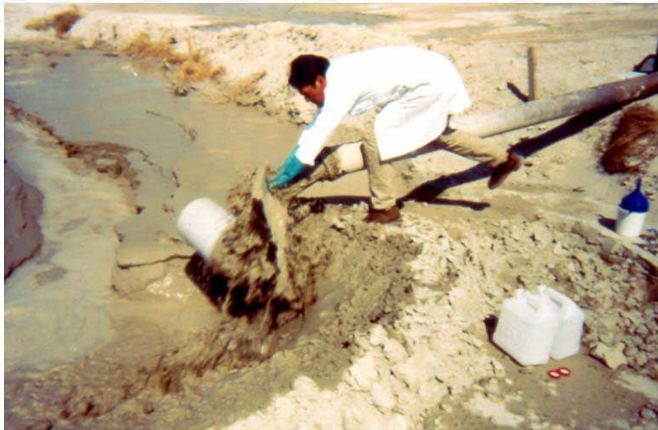
Fig. 1. Pipe used to transport the solid residuals until the jales dam
