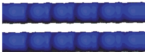
Fig. 16. The distribution of the electron charge for undamaged bilayer graphene (the density equals 0.4 \text{ el} / \text{\AA}^3 ).
