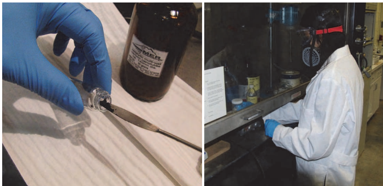
Fig. 4. Simple protection methods for using potentially hazardous engineered nanomaterials in laboratory conditions.
